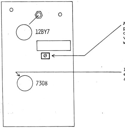
Adjust to 123 volts at the point indicated below. Use only a high impedance D.C. voltmeter. Allow 30 minutes warm-up before adjustment.
