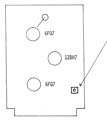
Adjust for lowest I.M. or / second harmonic distortion on either 4 or 8 ohm tap at 1 watt, then check at 10 watts. A change in the setting indicates a bad tube or component.
