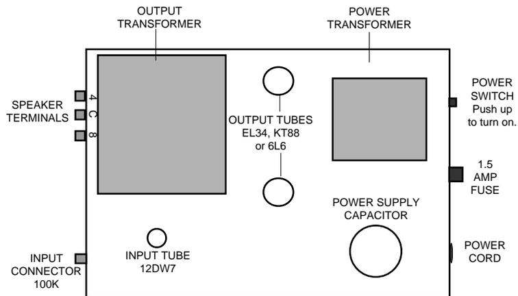
DIAGRAM ON THE BOTTOM OF THE AMPLIFIER:
